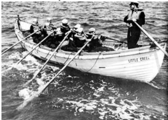
25 Foot Self bailing pulling boat Length 25'6", crew of 9 - 8 oars and coxswain
