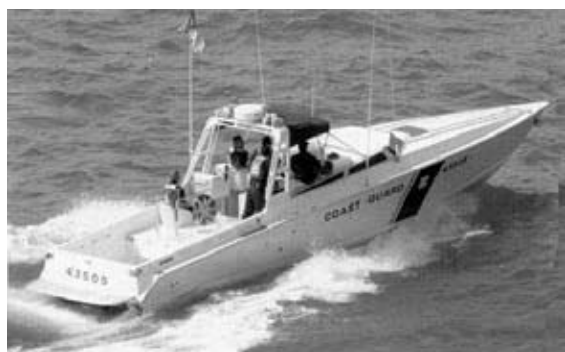
43 Foot FCI 43501 - 43505 Completed by April 1987 Length 43'6" x Beam 9'6" x Draft 3'3" 2 Caterpillar diesels 750 BHP Twin screw 39+ knots Designed and constructed by Tempest Marine for the Coast Guard. The boats are V-bottom monohull
