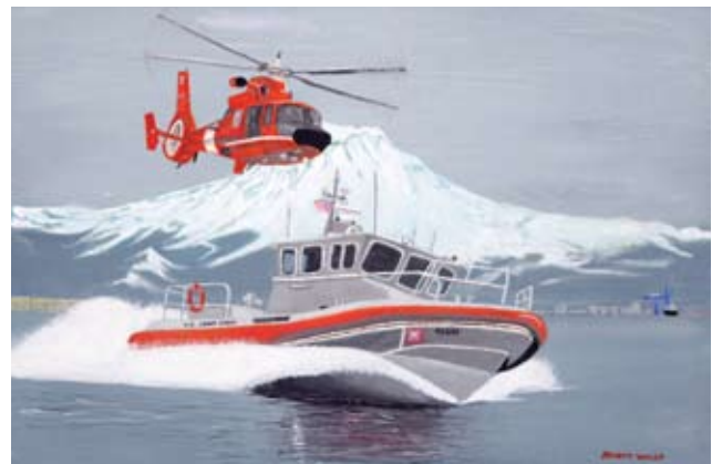
Response Boat at Commencement Bay by Marty Walsh. The response boat-medium (RB-M) is an all-aluminum, 45-foot boat with twin diesel engines and with water jet propulsion launched at Commencement Bay in Tacoma. Shown here with a HH-65 Dolphin helicopter, the RB-M, is the Coast Guard's newest boat to enter the fleet.
